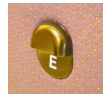
Aisle Light (LED)
